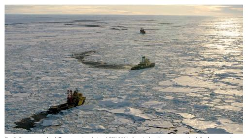
Fig. 2. To carry out the drilling operation during ACEX 2014, three icebreakers were required. Farthest away in the picture, the Russian nuclear powered icebreaker Sovetsky Soyuz is splitting the largest ice floes. The role of the Oden was to break up the medium-sized ice floes so that the icebreaker Vidar Viking (closest) could maintain its position with the drill string anchored in the seabed. Photo: Martin Jakobsson.
