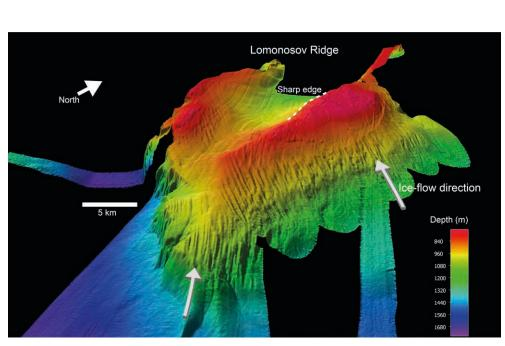
Fig. 5. Three-dimensional visualization of the crest of the Lomonosov Ridge showing where it was abraded by a kilometre-thick ice shelf. The image was created from measurements by multibeam echo sounder from the expedition on the Oden. The dotted line marks a sharp edge. The arrow to the right shows the direction in which the ice moved. See Fig. 1 for location on the Lomonosov Ridge.
